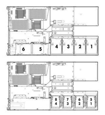
1-6 6 Non-hot plug LFF SATA or 4 Non-hot plug LFF SAS hard drive bays - Using quick release carrier.
