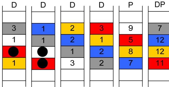
After RAID-DP has recreated a missing diagonal block, the process again switches to recreating a missing horizontal block from row parity. When the missing diagonal block in the gold diagonal has been recreated, enough information is available to recreate the missing horizontal block from row parity, as evident in the following diagram.
