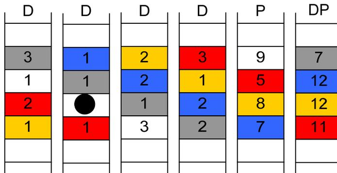
Once again, after the recovery of a diagonal block the process switches back to row parity, as it has enough information to recreate data for the one horizontal block. The final diagram in the double disk failure scenario follows next, with all data having been recreated with RAID-DP.
