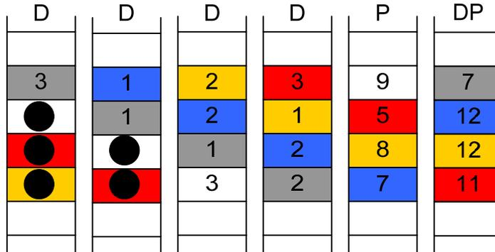
Once again, after RAID-DP has recovered a missing diagonal block in a diagonal stripe, enough information exists for row parity to recreate the one missing horizontal block in the first column, as illustrated in the next diagram.
