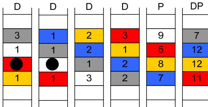
After the missing block in the horizontal row has been recreated, reconstruction switches back to diagonal parity to recreate a missing diagonal block. RAID-DP can continue in the current chain on the red diagonal stripe, as shown in the next diagram.
