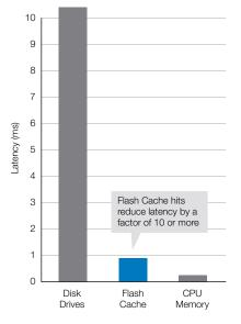
Latency is typically 10ms or higher when accessing data from disk drives. Flash Cache modules reduce latency by a factor of 10 or more compared to disk drives when there is a cache hit.
